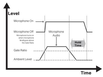
Figure 3.29. PSR1212 automixing gate functions
